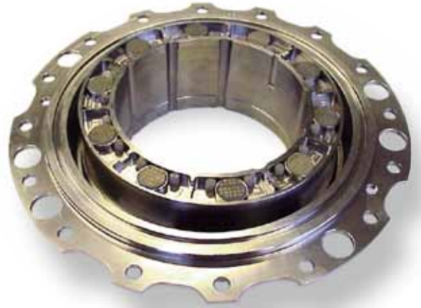
Photo 2: Telemetry system assembly for taking measured data from HP compressor and turbine rotor (42 ch. dyn. S/G and 24 ch. T/C)
