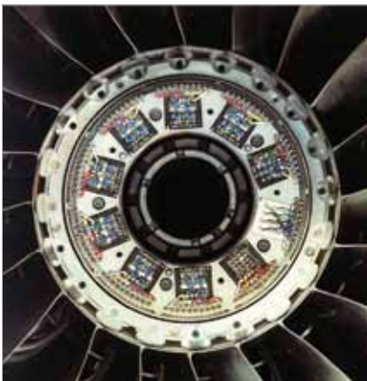
Photo 1: Telemetry installation for LP compressor test on El200 engine
