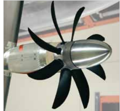
Photo 4: Propeller model with strain gage balance and telemetric data transmission
