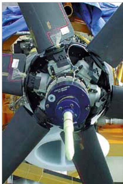
Photo 3: Telemetry transmitter unit mounted on propeller hub
