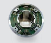
Customized 16ch telemetry for installation inside electric motor
