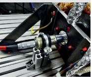
8ch telemetry on electric motor test rig (end of shaft installation)
