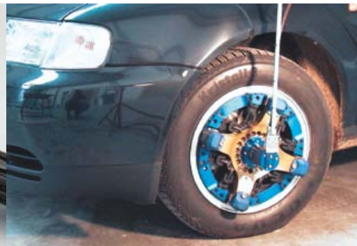
6-component wheel force transducer with telemetric data transmission
