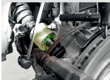
Torque measurement system installed on drive shaft
