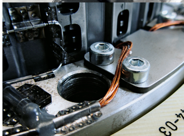
Instrumented clutch assembly prepared for temperature measurement
