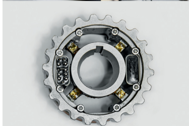
Modified pulley with telemetry for torque measurement
