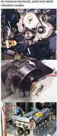
measurement on an A/C compressor
