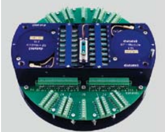
16 channel telemetry transmitter with patch panel and S/G bridge completion cards
