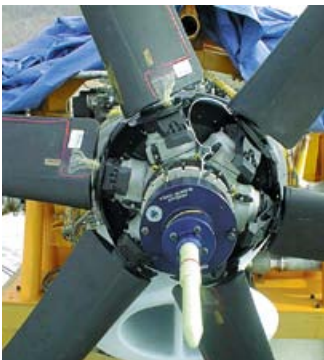
Telemetry transmitter unit mounted on the propeller hub
