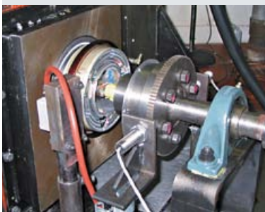
Multi-axis vibration measurement on marine engine timing gear test rig
