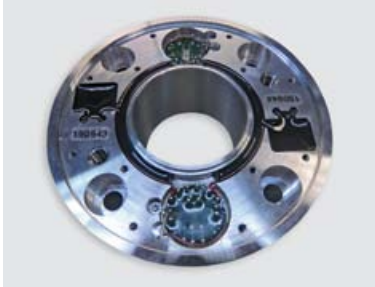
Telemetry for torsional vibration measurement on gear wheel test rig
