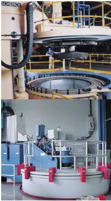
Spin test facilities equipped with telemetry for turbine rotor testing
