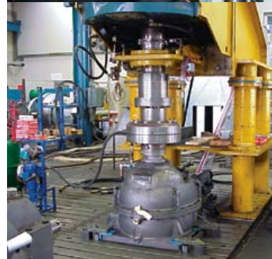
Torque measurement on pump test rig
