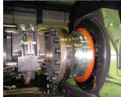
Telemetry system for testing of torque, angular position and temperature on an automotive clutch test rig
