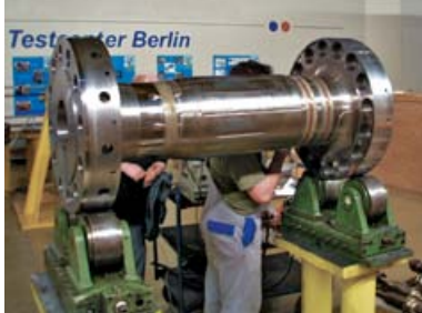
Load coupling for torque measurement on heavy-duty gas turbine test rig
