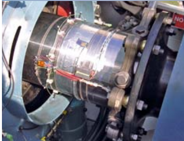
Torque survey on a wind turbine generator shaft (short-term installation)
