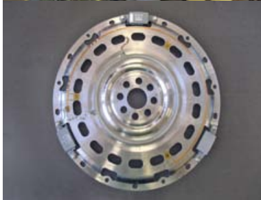
Automotive flex plate modified for engine torque measurement
