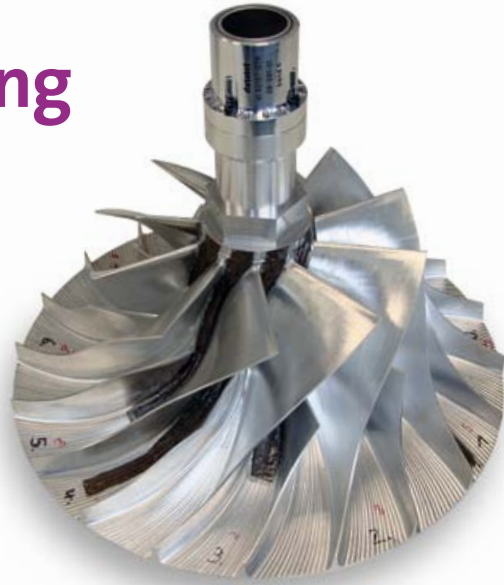
Instrumented Compressor Rotor
