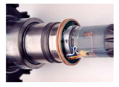
Torque Measurement in Automotive Transmissions
